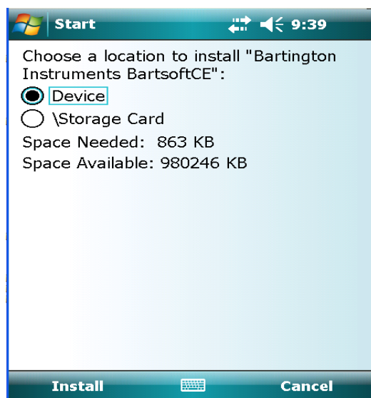
Image 1: If there is a Storage Card on the device then the user is prompted to choose where to install the application.
